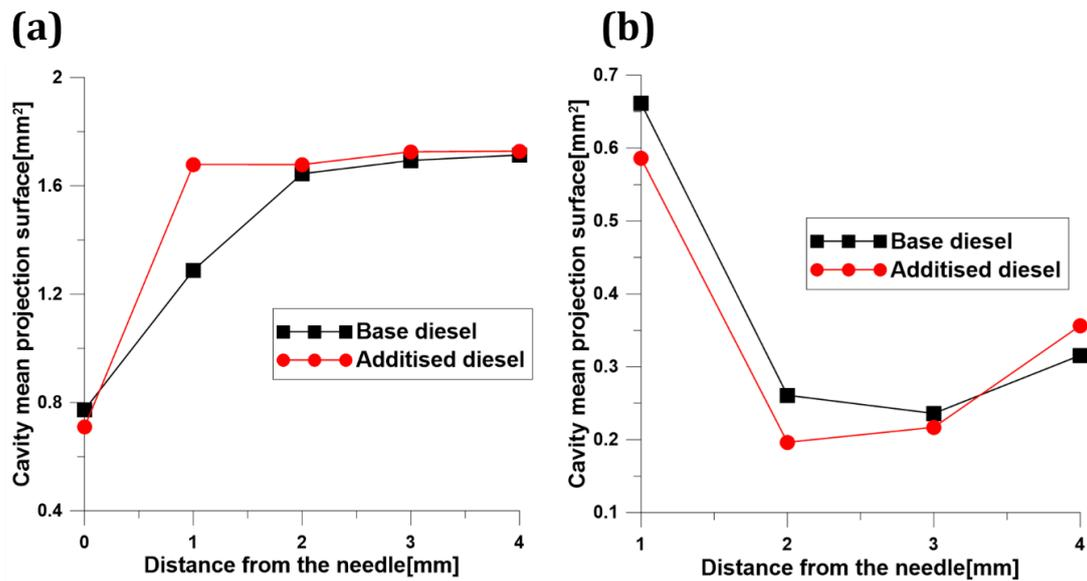
Figure 24: Mean projection surface in  $\text{mm}^2$  for two types of diesel (base and additised) and for (a)  $CN=7.7$ ,  $Re=35500$  and  $NL=0.5\text{mm}$  and (b)  $CN=4.0$ ,  $Re=35500$  and  $NL=1\text{mm}$ . The two different trends are attributed to the different behaviour of the additised diesel in respect to different main forms of cavitation
