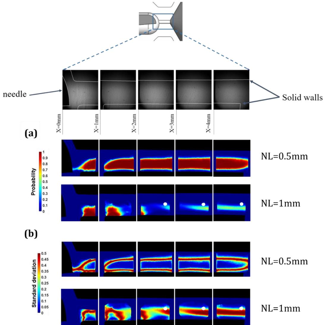
Figure 1: (a) Mean and (b) standard deviation images two different needle lifts (NL), with same CN and Re (CN=4.0, Re=35500)
