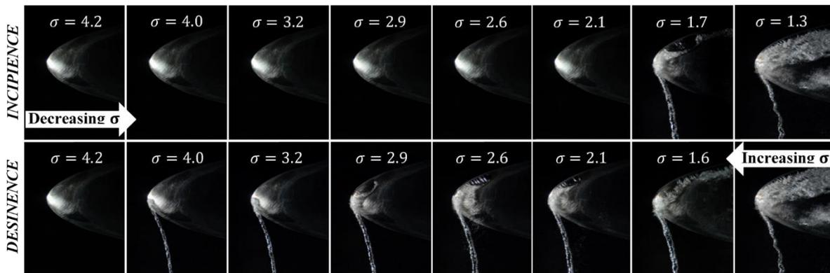
Figure 1: A typical tip vortex cavitation inception-desinence test, performed at 10 m/s and 12° of incidence angle. The large difference between the two thresholds results in the so-called hysteresis problem. For this test, water was fully saturated with air at 18° Celsius.
