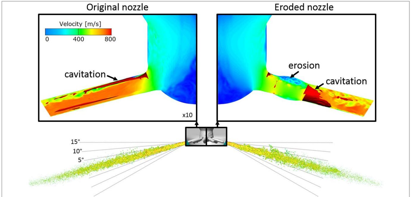
Comparison between simulation results between the original and the eroded nozzle. Internal nozzle flow presented with velocity cut and vapor iso-surfaces and spray visualizations.
