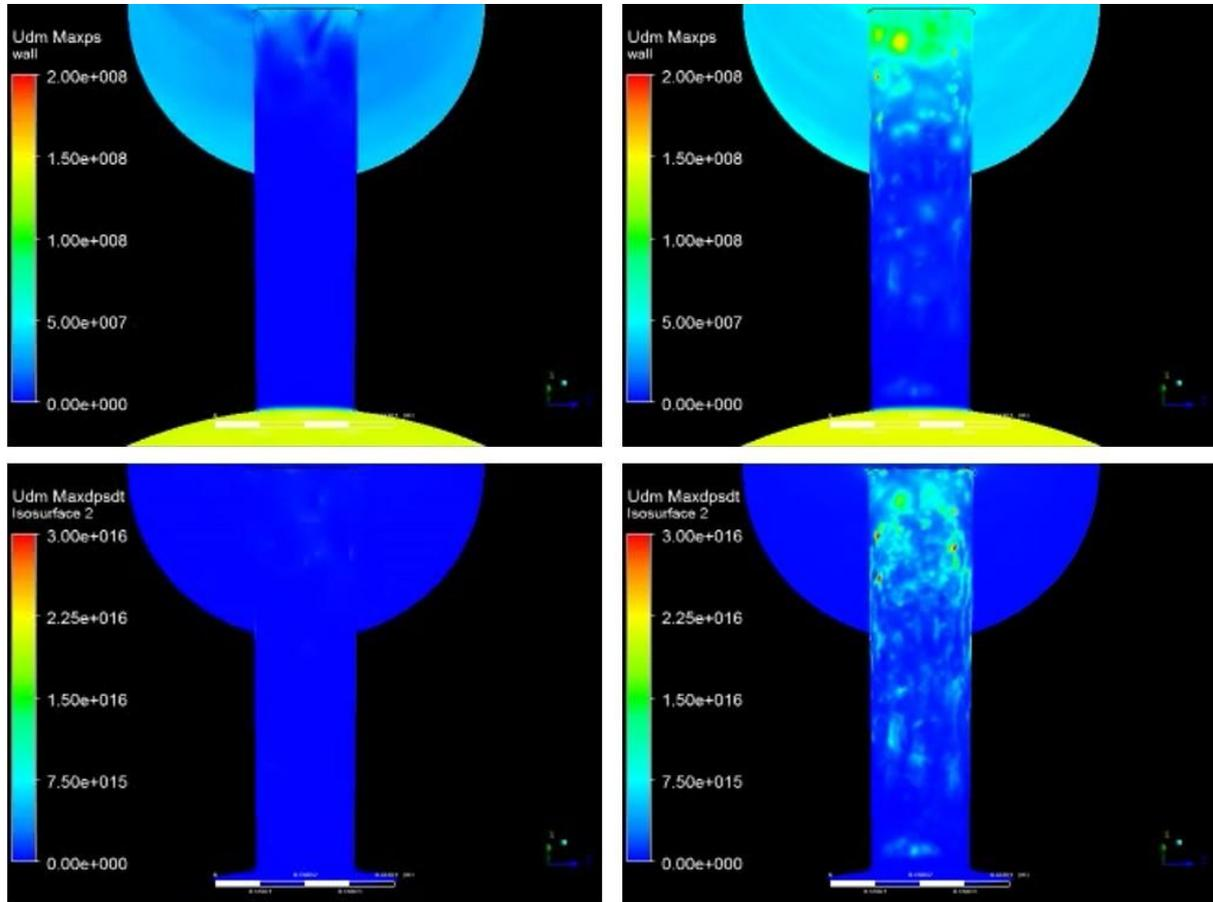
CFD results from a cavitating flow inside a control orifice in a prototype diesel injector. Accumulation of maximum pressure (top, 0 to  $2e8$  Pa) and rate of pressure change (bottom, 0 to  $3e16$  Pa/s) over  $10\mu s$  (left is at time 0). Maxima correlates well with the location of damage on hardware.
