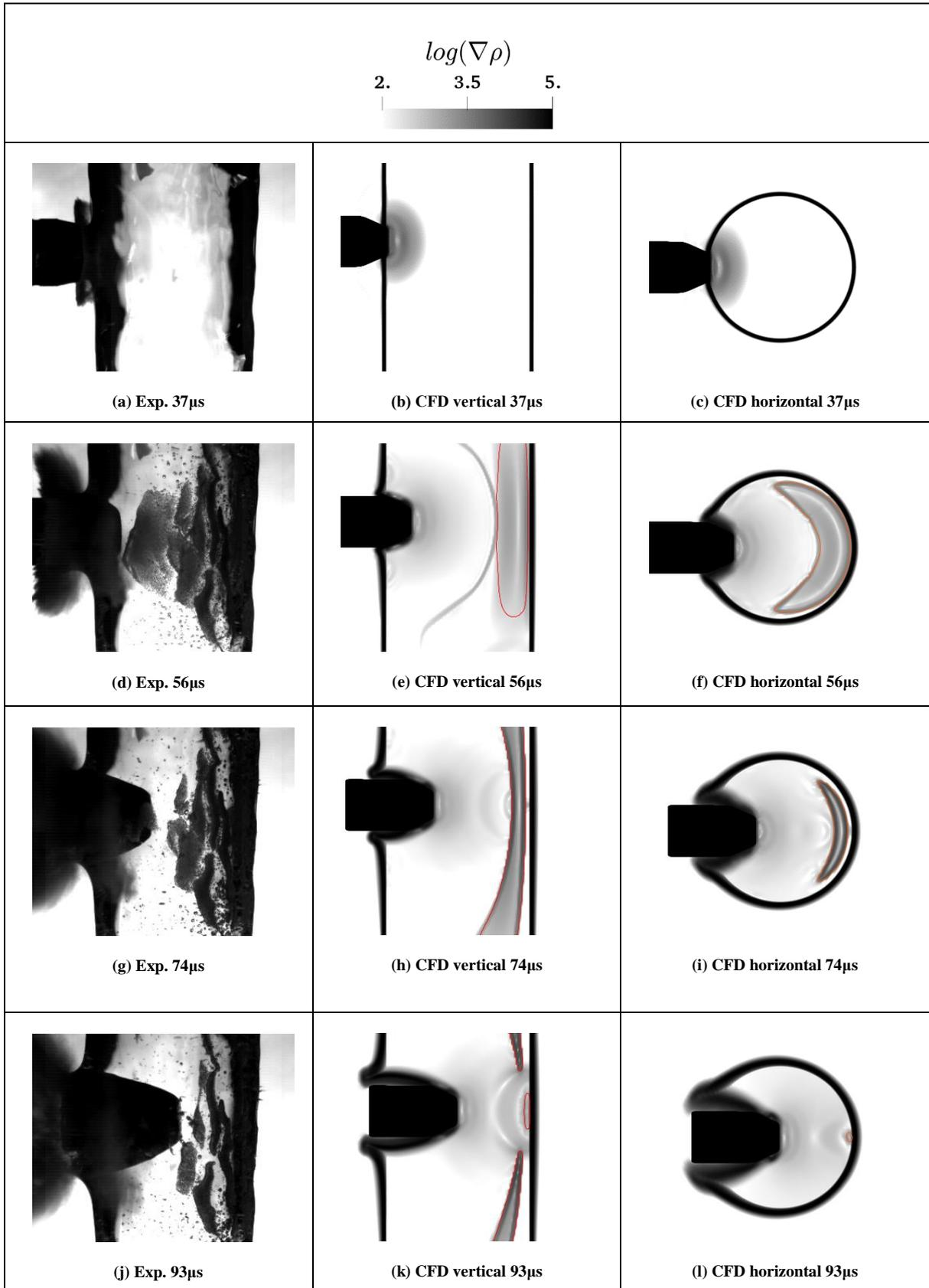
Consecutive frames from the experimental data from Field et al. (left) and numerical results (middle, right) for the impact of projectile on water jet, with  $U_{\text{impact}}=210\text{m/s}$ . For the CFD results, the logarithm of the magnitude of the gradient of density is plotted on the vertical (middle) and horizontal (right) middle plane on grayscale, along with the 0.1% contour for vapour volume fraction, represented by a red line
