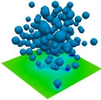
Representation of a cavity cloud as a cluster of Lagrangian bubbles
