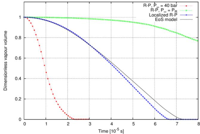
Time history of bubble cloud volume using Lagrangian model with different forms of the Rayleigh-Plesset equation
