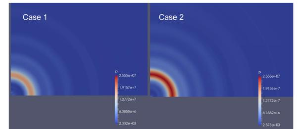
Figure 2. Pressure pulses produced by two bubbles with different collapse rates
