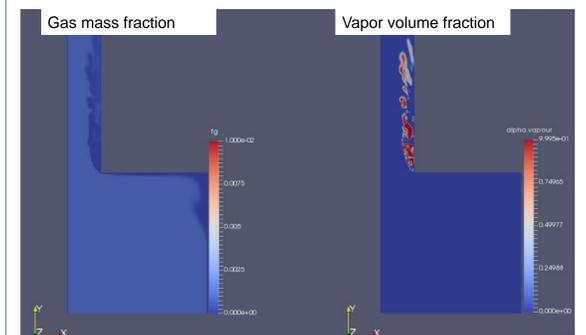
Figure 3. distribution of gas mass fraction and vapor volume fraction after 6.ms
