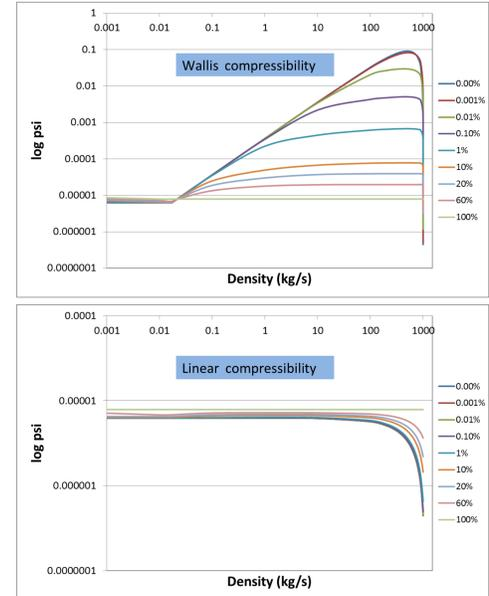
Figure 2. compressibility vs density relation with Wallis and linear compressibility model
