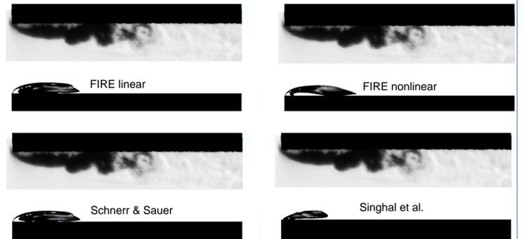
Figure 4. Vapor cloud in a throttle flow with different R-P cavitation models
