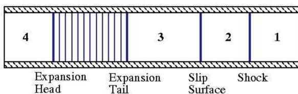
Figure 1. Flow configuration of a shock tube [3]
