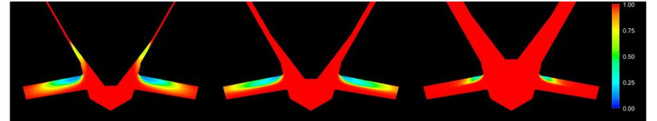
Fig. 3- Mid-plane view of the CFD at three fixed lifts. The scale shows liquid phase volume fraction. 800 bar upstream and 50 bar downstream.
