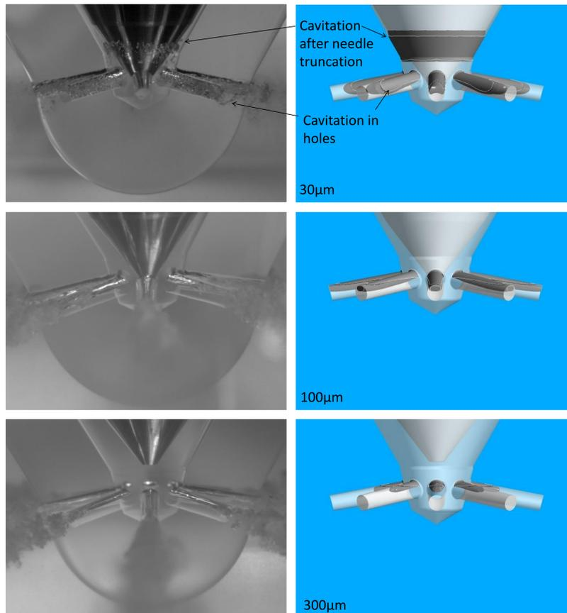
Fig. 2- LSM and equivalent CFD showing cavitation at three fixed valve lifts. 800 bar upstream and 50 bar downstream (equivalent). The CFD shows isosurface of 90% liquid volume fraction.
