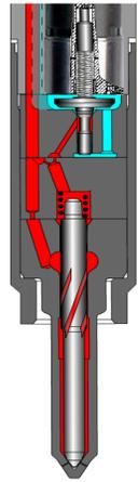
Fig. 1- Typical diesel injector. The red areas indicate HP fuel flow paths.
