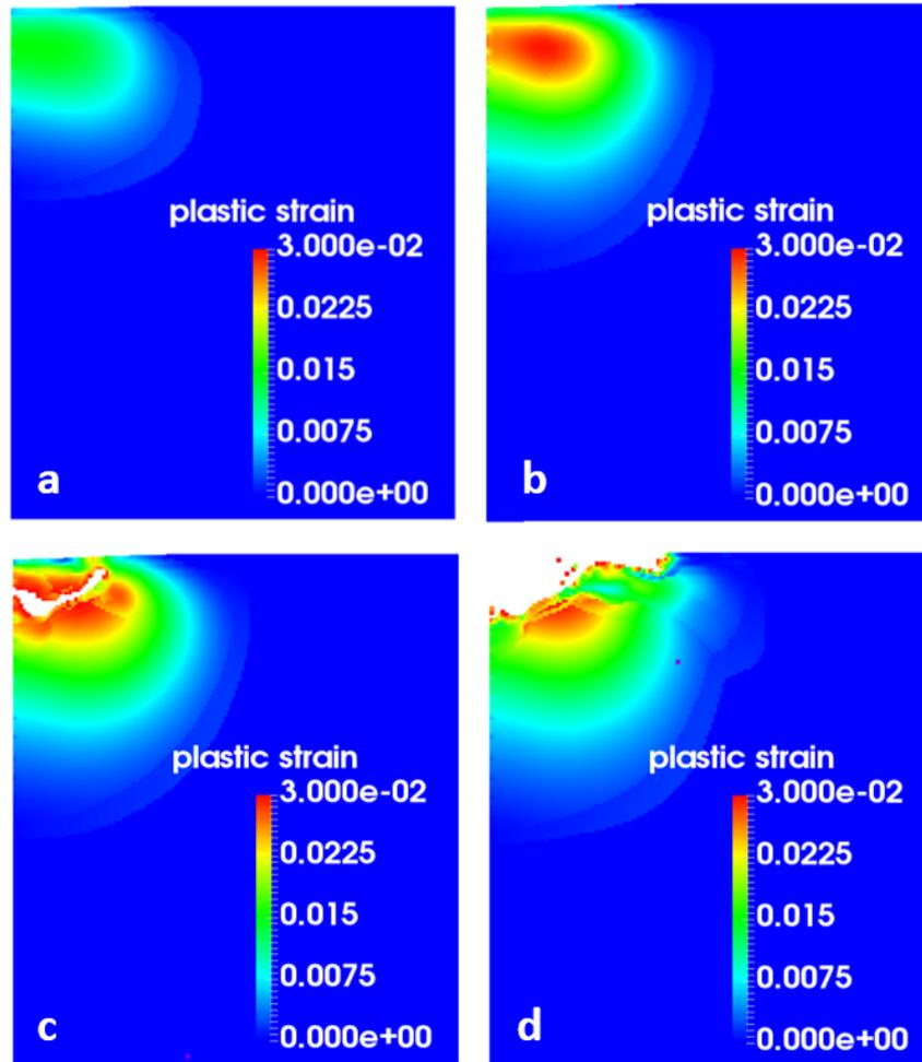
*Sequence of images from 2D axisymmetric damage simulation of a stainless steel A-2205 specimen under spherical indentation, (a) Shows the plastic strain accumulation in material without damage, (b) Shows high plastic strain zone just beneath the top surface, (c) damage initiation from the point of highest plastic strain, (d) Material loss due to a single indent.*
