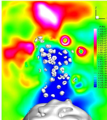
Pressure and vapor structures between the primal and first rebound collapses, middle slice in y-z plane. Non-spherical focused collapse of individual bubbles and large vapor region at the wall. The bubble deformation is characterized by induced jets pointing towards the cloud center.
